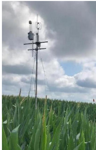
Southwest Sciences gas monitor
